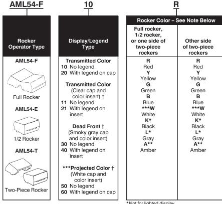
NOTE: AML54-F10 and AML54-F20 are one-piece, one-color full rockers. Thus only one color code letter is necessary when ordering. Include a two letter code for all other AML54-E (and AML54-T) catalog listings.
