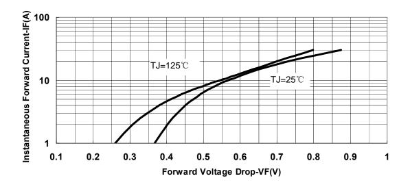
Fig.3-Typical Instantaneous Forward Voltage Characteristics
