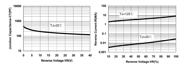
Fig.1-Typical Junction Capacitance
