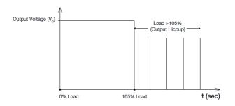
Additionally, if the  $I_{\rm O}$  is <130% but >110% for a prolong period of time (depending on the load), the Over Temperature Protection (OTP) will be activated due to high temperature on critical components. The power supply will then go into hiccup mode until the fault is removed; and, the input voltage is removed, then reapplied.
