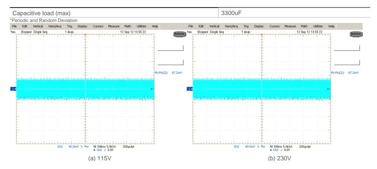
Fig. 2 Ripple & Noise example, 20MHz BW
