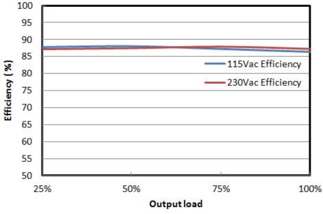
Fig.1 Efficiency versus output load
