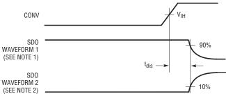
NOTE 1: WAVEFORM 1 IS FOR AN OUTPUT WITH INTERNAL CONDITIONS SUCH THAT THE OUTPUT IS HIGH UNLESS DISABLED BY THE OUTPUT CONTROL NOTE 2: WAVEFORM 2 IS FOR AN OUTPUT WITH INTERNAL CONDITIONS SUCH THAT THE OUTPUT IS LOW UNLESS DISABLED BY THE OUTPUT CONTROL 18645 TODS
