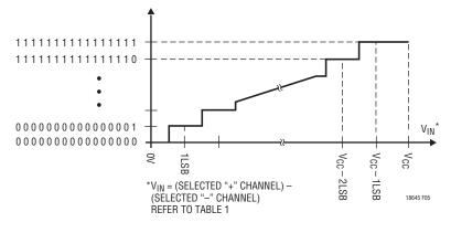
Figure 5. LTC1865 Transfer Curve
