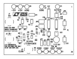
Component Side Silk Screen for LTC1864 Evaluation Circuit
