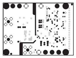
Ground Layer with Separate Analog and Digital Grounds
