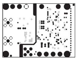
Supply Layer with 5V Digital Supply and Analog Ground Repeated
