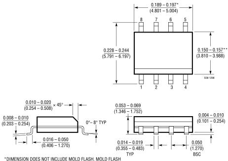
\*DIMENSION DOES NOT INCLUDE MOLD FLASH. MOLD FLASH SHALL NOT EXCEED 0.006" (0.152mm) PER SIDE \*\*DIMENSION DOES NOT INCLUDE INTERLEAD FLASH. INTERLEAD
