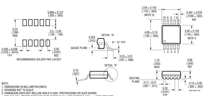
**MS** Package **10-Lead Plastic MSOP** (Reference LTC DWG # 05-08-1661)
