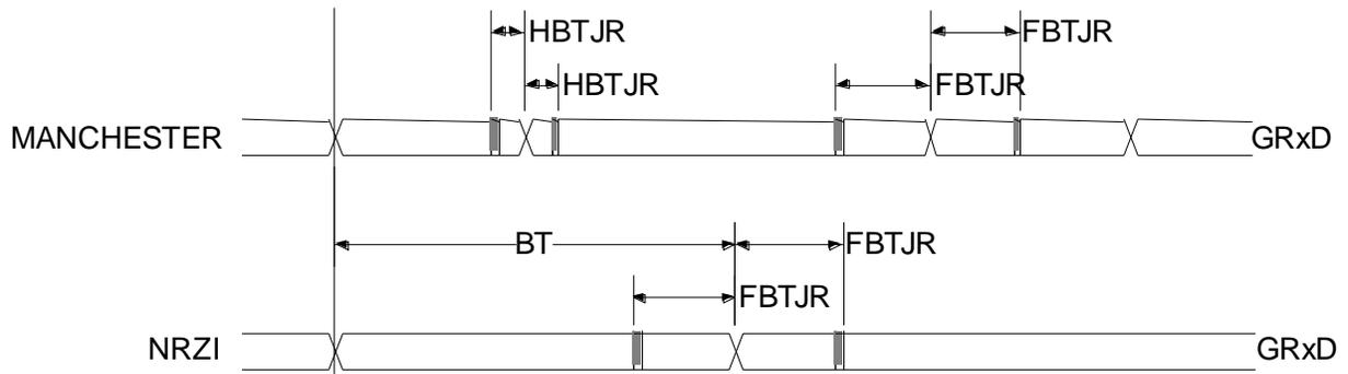
Figure 11. GSC Receiver Timings (Internal Baud Rate Generator)
