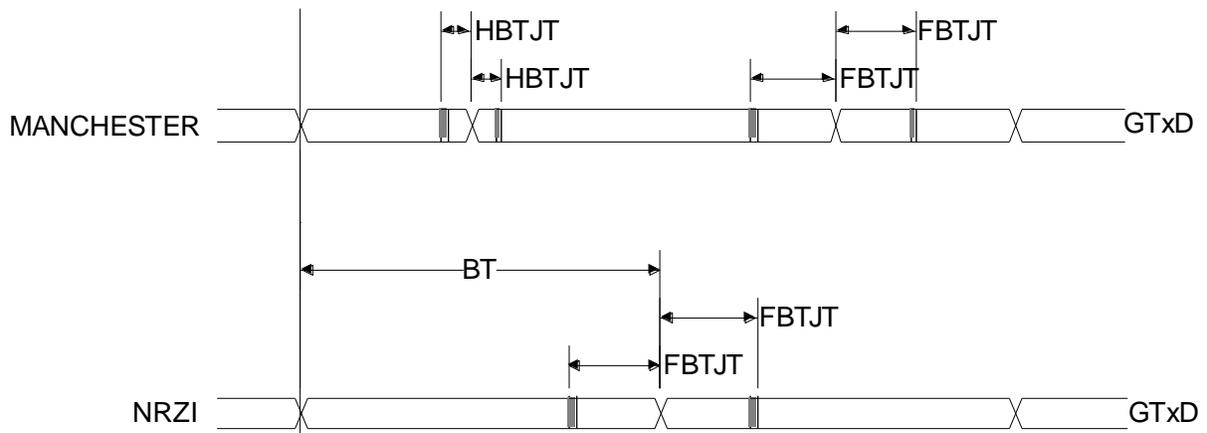
Figure 12. GSC Transmit Timings (Internal Baud Rate Generator)
