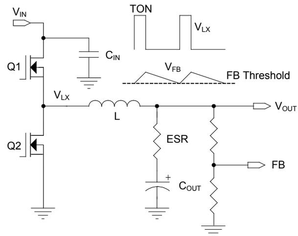
**Figure 1 — PWM Control Method,  $V_{OUT}$  Ripple**
