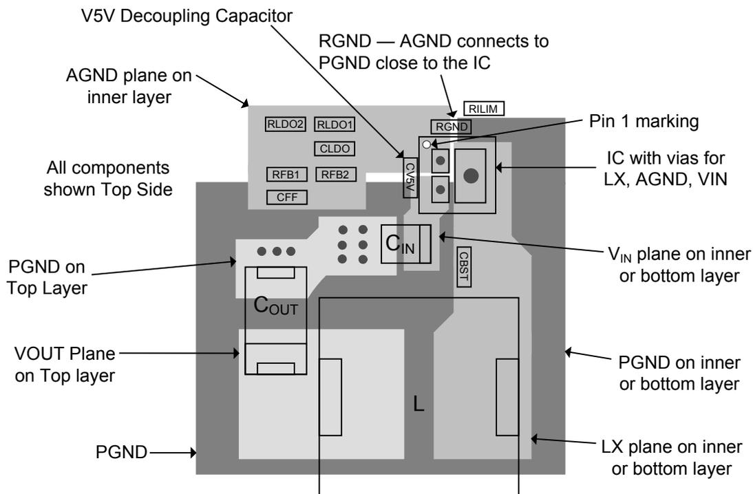
Figure 15 — PCB Layout
