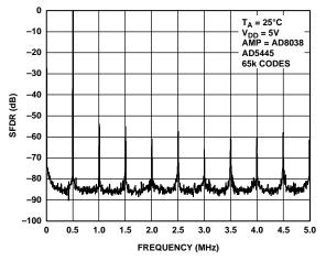
Figure 39. Wideband SFDR,  $f_{OUT} = 500 \text{ kHz}$ , Clock = 10 MHz
