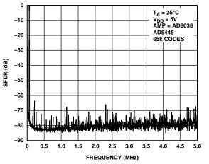
Figure 40. Wideband SFDR,  $f_{OUT} = 50 \text{ kHz}$ , Clock = 10 MHz
