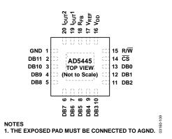
Figure 8. AD5445 Pin Configuration (LFCSP)
