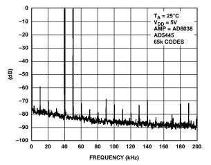
Figure 47. Wideband IMD,  $f_{OUT} = 60 \text{ kHz}$ , 50 kHz, Clock = 10 MHz
