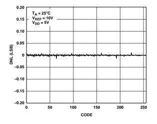
Figure 12. DNL vs. Code (8-Bit DAC)
