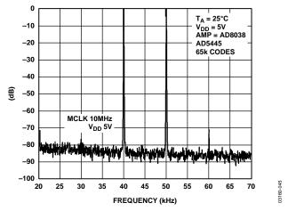
Figure 45. Narrow-Band IMD,  $f_{OUT} = 40 \text{ kHz}$ , 50 kHz, Clock = 10 MHz
