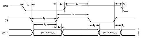
Figure 2. Timing Diagram
