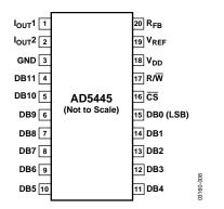
Figure 7. AD5445 Pin Configuration (TSSOP)
