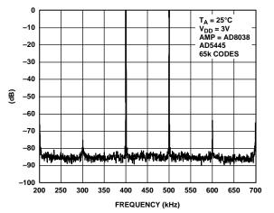
Figure 43. Narrow-Band IMD,  $f_{OUT} = 400 \text{ kHz}$ , 500 kHz, Clock = 10 MHz
