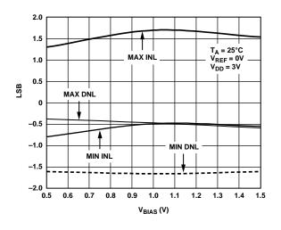
Figure 18. Linearity vs. V<sub>BIAS</sub> Voltage Applied to I<sub>OUT</sub>2, AD5445
