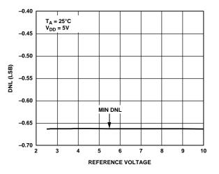
Figure 16. DNL vs. Reference Voltage, AD5445
