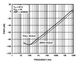
Figure 34. Power Supply Rejection vs. Frequency
