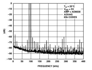
Figure 46. Wideband IMD,  $f_{OUT} = 90 \text{ kHz}$ , 100 kHz, Clock = 25 MHz
