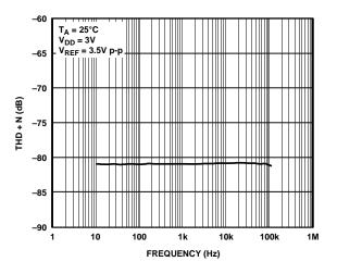
Figure 35. THD and Noise vs. Frequency
