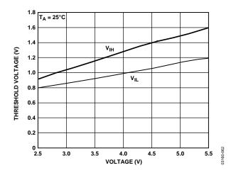
Figure 33. Threshold Voltages vs. Supply Voltage
