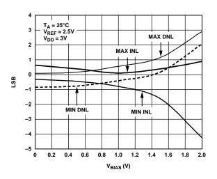
Figure 19. Linearity vs. V<sub>BIAS</sub> Voltage Applied to I<sub>OUT</sub>2, AD5445
