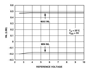
Figure 15. INL vs. Reference Voltage, AD5445
