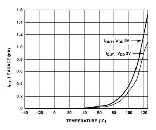
Figure 25. Iou 1 Leakage Current vs. Temperature
