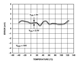
Figure 17. Gain Error vs. Temperature
