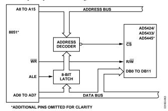
Figure 56. 8xC51-to-AD5424/AD5433/AD5445 Interface
