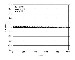
Figure 13. DNL vs. Code (10-Bit DAC)
