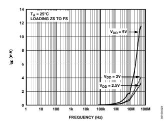
Figure 27. Supply Current vs. Update Rate
