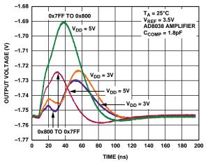
Figure 32. Midscale Transition,  $V_{REF} = 3.5 V$
