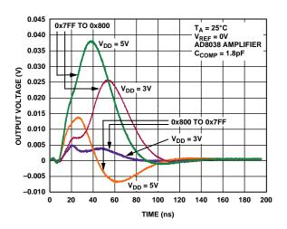
Figure 31. Midscale Transition,  $V_{REF} = 0 V$
