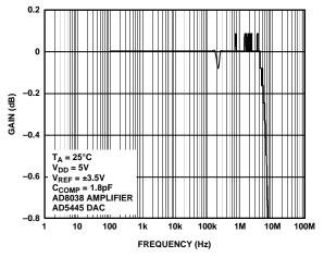
Figure 29. Reference Multiplying Bandwidth—All 1s Loaded
