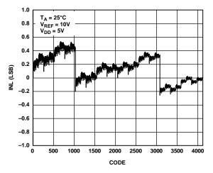
Figure 11. INL vs. Code (12-Bit DAC)
