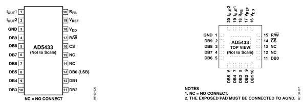
Figure 5. AD5433 Pin Configuration (TSSOP)
