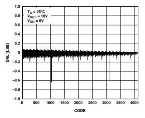
Figure 14. DNL vs. Code (12-Bit DAC)
