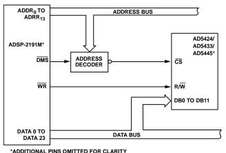
Figure 55. ADSP-2191M-to-AD5424/AD5433/AD5445 Interface
