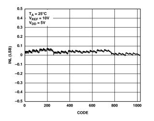
Figure 10. INL vs. Code (10-Bit DAC)
