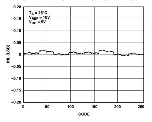
Figure 9. INL vs. Code (8-Bit DAC)
