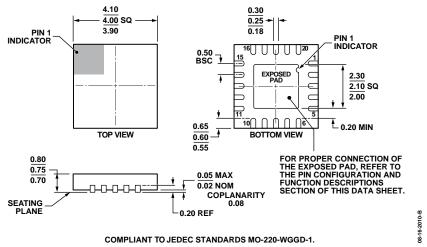
Figure 60. 20-Lead Lead Frame Chip Scale Package [LFCSP\_WQ] 4 mm × 4 mm Body, Very Thin Quad (CP-20-6) Dimensions shown in millimeters
