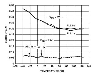
Figure 26. Supply Current vs. Temperature
