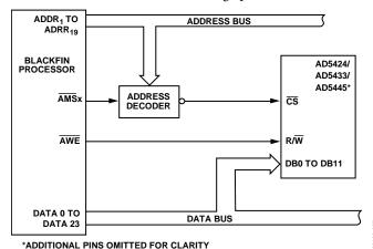
Figure 57. Blackfin Processor-to-AD5424/AD5433/AD5445 Interface
