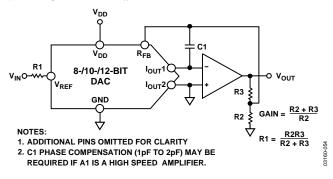
Figure 53. Increasing the Gain of the Current Output DAC
