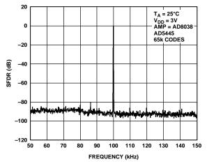
Figure 42. Narrow-Band SFDR,  $f_{OUT} = 100 \text{ kHz}$ , MCLK = 25 MHz
