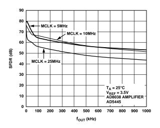
Figure 37. Wideband SFDR vs. fout Frequency
