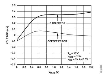
Figure 21. Gain and Offset Errors vs. VBIAS Voltage Applied to IOUT2
