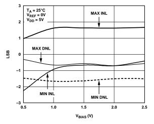
Figure 22. Linearity vs. V<sub>BIAS</sub> Voltage Applied to I<sub>OUT</sub>2, AD5445
