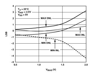
Figure 23. Linearity vs. V<sub>BIAS</sub> Voltage Applied to I<sub>OUT</sub>2, AD5445
