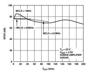
Figure 36. Wideband SFDR vs. fout Frequency
