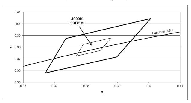
Figure 11: Graph of Neutral White Test Bins in xy Color Space (Pulsed Test Conditions,  $T_i = 25^{\circ}C$ )
