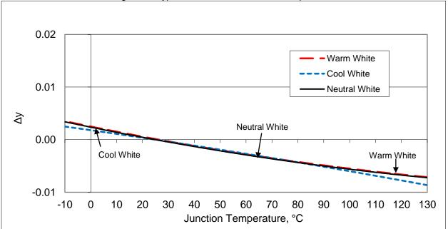
Figure 4: Typical ccx Shift vs. Junction Temperature
