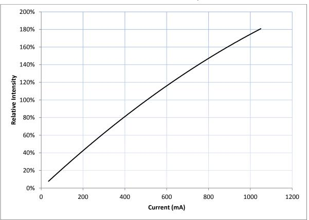
Figure 2: Typical Flux vs. Current,  $T_j = 25^{\circ}C$
