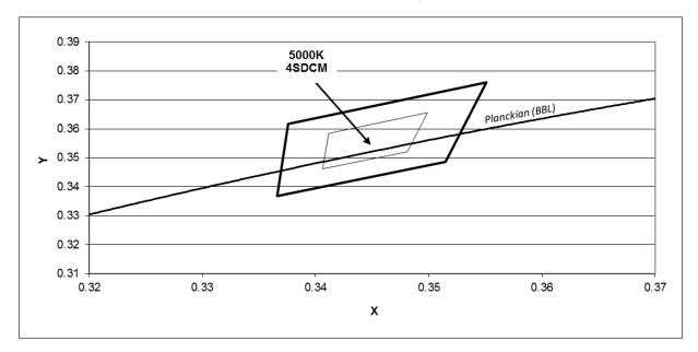
Figure 12: Graph of Cool White Test Bins in xy Color Space (Pulsed Test Conditions,  $T_j = 25^{\circ}C$ )
