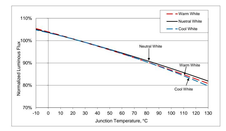
Figure 3: Typical Flux vs. Junction Temperature
