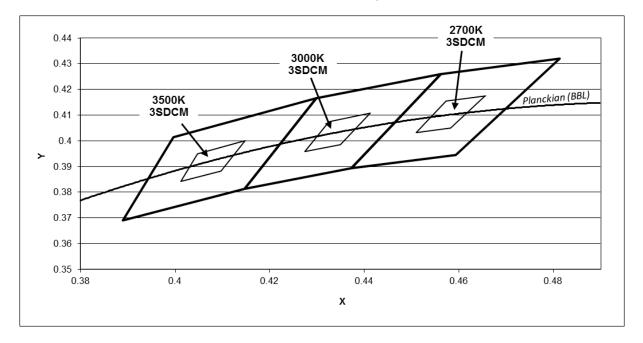
Figure 10: Graph of Warm White Test Bins in xy Color Space (Pulsed Test Conditions,  $T_j = 25^{\circ}C$ )
