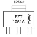
FZT 1051A = Product Type Marking Code YWW = Date Code Marking Y or  $\overline{Y}$  = Last Digit of Year (ex: 5= 2015) WW or  $\overline{W}W$  = Week Code (01~53)
