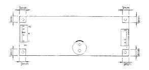
Please leave 4mm space from the surfaces and the sides of PCB, especially from the solder surface, 8mm space is necessary. If the space is not enough, the specification of insulation and withstand will not be satisfied.
