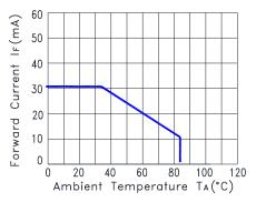
Fig.2 Forward Current Derating Curve
