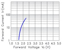
Fig.3 Forward Current vs. Forward Voltage
