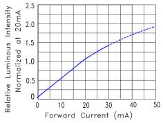
Fig.4 Relative Luminous Intensity vs. Forward Current
