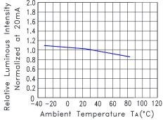
Fig.5 Relative Luminous Intensity VS. Ambient Temperature
