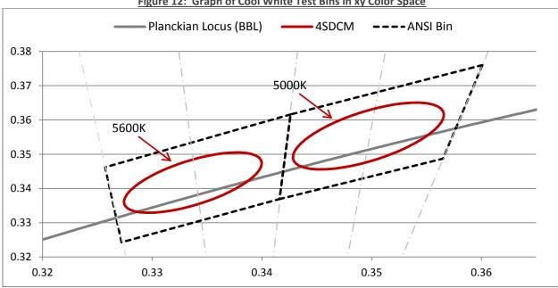
Figure 12: Graph of Cool White Test Bins in xy Color Space
