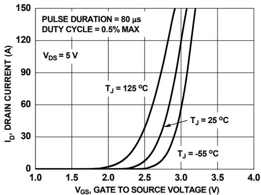
Figure 5. Transfer Characteristics
