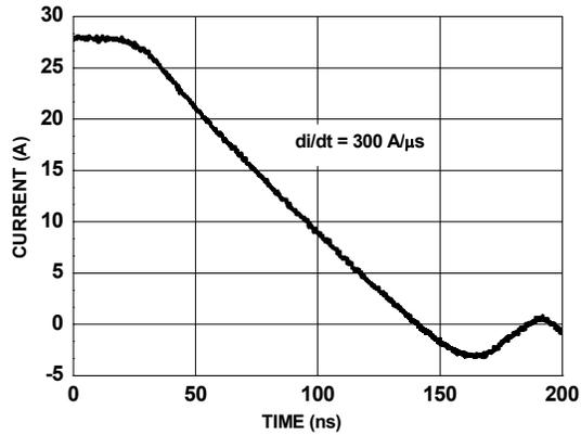
Figure 14. FDMS7658AS SyncFET<sup>™</sup> Body Diode Reverse Recovery Characteristic
