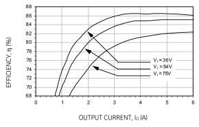
Figure 13. Converter Efficiency versus Output Current.
