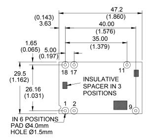
Through-Hole Pad Layout – Component side view
