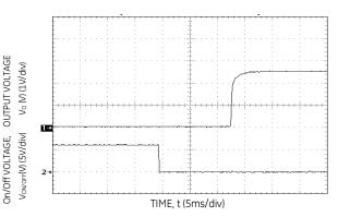
Figure 18. Typical Start-Up Using Remote On/Off, negative logic version shown.
