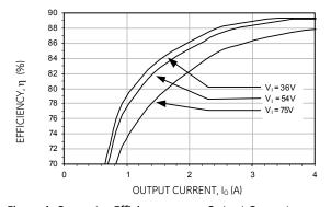
Figure 1. Converter Efficiency versus Output Current
