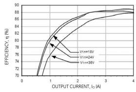
Figure 49. Converter Efficiency versus Output Current.
