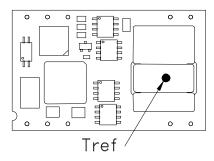
Figure 66. T<sub>ref</sub> Temperature Measurement Location.
