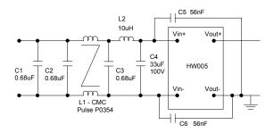
Figure 67. Suggested Configuration for EN55022 Class R
