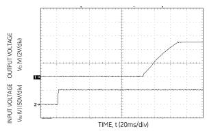
Figure 5. Typical Start-Up with application of Vin.
