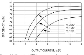
Figure 37. Converter Efficiency versus Output Current.
