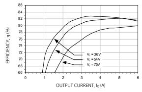
Figure 25. Converter Efficiency versus Output Current
