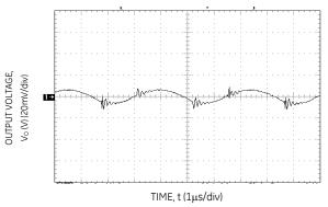
Figure 26. Typical Output Ripple and Noise.
