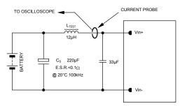
NOTE: Measure input reflected ripple current with a simulated source inductance (L<sub>TEST</sub>) of 12μH. Capacitor C<sub>S</sub> offsets possible battery impedance. Measure current as shown above
