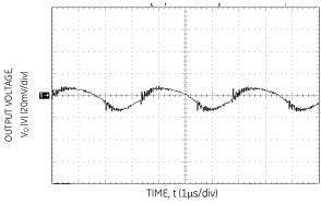
Figure 2. Typical Output Ripple and Noise.
