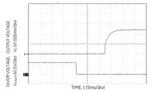
Figure 42. Typical Start-Up Using Remote On/Off, negative logic version shown.
