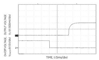
Figure 45. Transient Response to Dynamic Load Change from 50% to 75% to 50% of full load.
