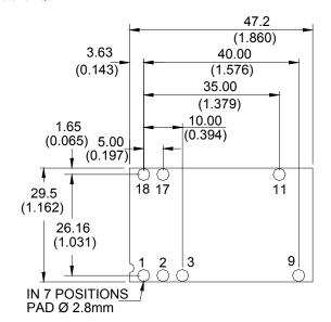
Surface Mount Pad Layout - Component side view
