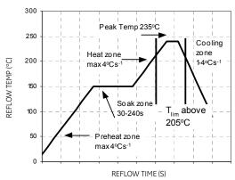
Figure 72. Recommended Reflow Profile
