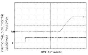
Figure 53. Typical Start-Up with application of Vin.
