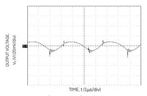
Figure 38. Typical Output Ripple and Noise.
