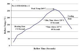
Figure 74. Recommended linear reflow profile using Sn/Aq/Cu solder.
