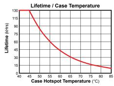
The area under the life-temperature curve represents where the driver has highly reliable operation within specification. Driver performance may drift out of published specifications as the hours of operation exceed the curve at a given temperature. Higher operating temperatures increase the chances of a failure to function. Other electrical, mechanical and environmental factors affect driver lifetime but are not represented in this calculation.
