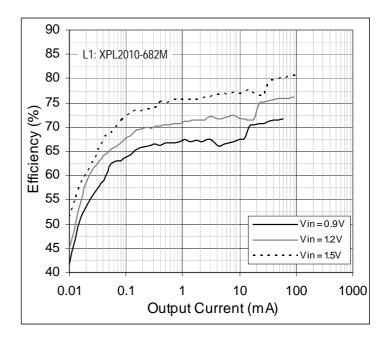
Figure 8: Efficiency vs. Output Current; V<sub>OUT</sub> = 1.8V
