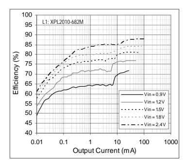
Figure 10: Efficiency vs. Output Current; V<sub>OUT</sub> = 3.0V
