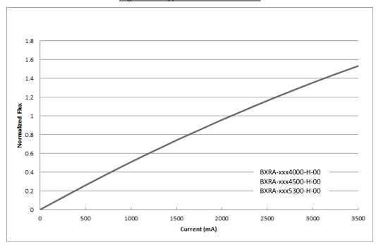
Figure 7: Typical Flux vs. Current
