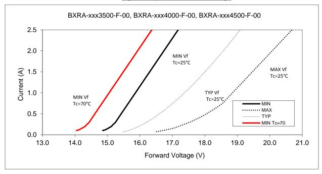
Figure 3: Typical Current vs. Voltage
