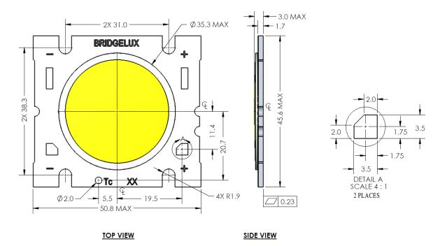
Figure 14: Drawing for RS Arrays
