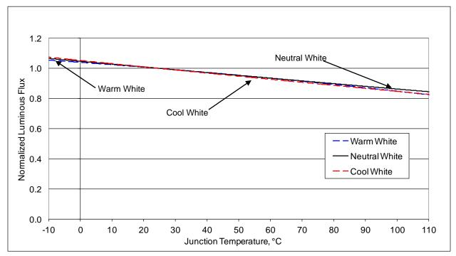
Figure 8: Typical Flux vs. Junction Temperature
