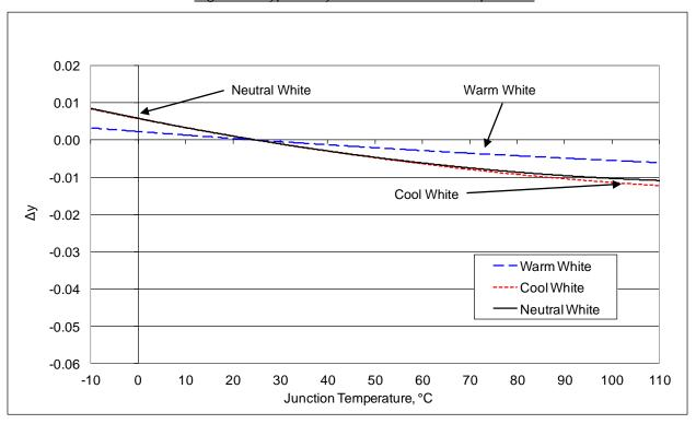
Figure 10: Typical ccx Shift vs. Junction Temperature
