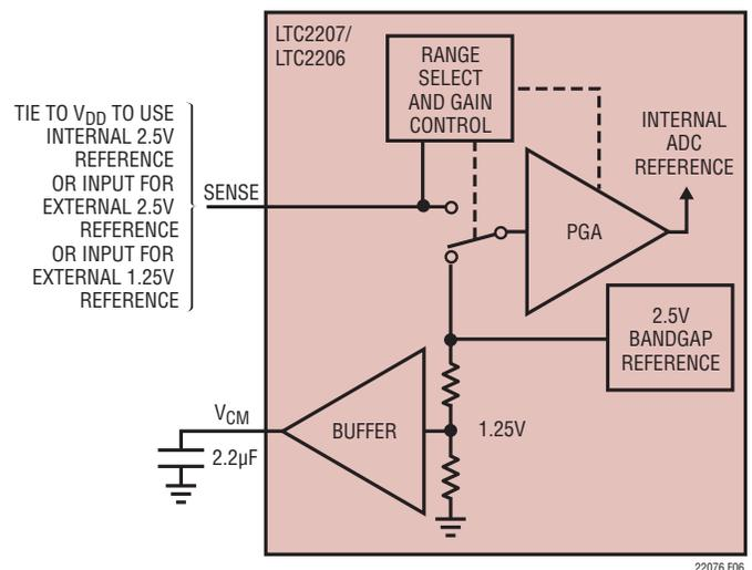
Figure 6. Reference Circuit
