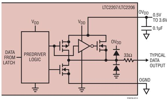
Figure 11. Equivalent Circuit for a Digital Output Buffer
