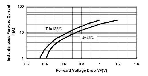
Fig.3-Typical Instantaneous Forward Voltage Characteristics
