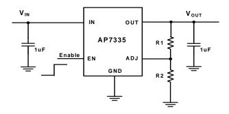
The output voltage is calculated by:
