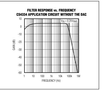
Figure 16. Filter Response of CS4334 Filter Configuration
