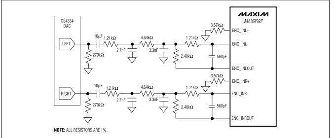
Figure 15. Lowpass Filter Configuration for the Cirrus CS4334
