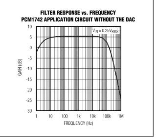
Figure 14. Filter Response of PCM1742 Filter Configuration
