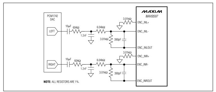
Figure 13. Lowpass Filter Configuration for the Burr-Brown PCM1742
