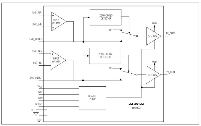
Figure 1. MAX9597 Audio Section Functional Diagram
