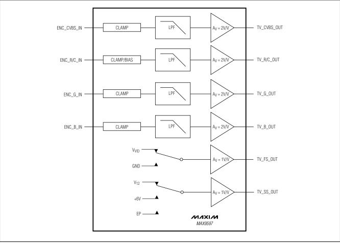
Figure 3. MAX9597 Video Section Function Diagram
