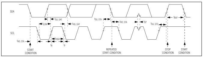
Figure 4. I<sup>2</sup>C Serial-Interface Timing Diagram
