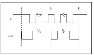
Figure 5. START, STOP, and REPEATED START Conditions
