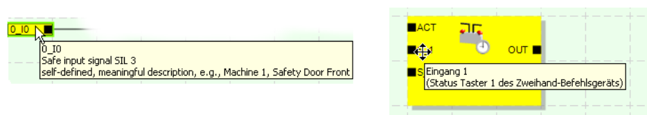
Figure 2-9 Examples of tool tips in the connection editor in offline mode (while editing the safety logic)
