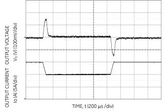
Figure 9. Transient Response to Dynamic Load Change, 0.1A/ $\mu$ S, from 75% to 50% to 75% of full load.
