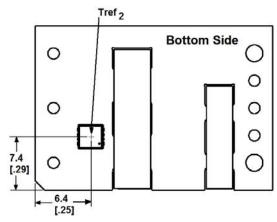
Figure 19. Tref<sub>x</sub> Temperature Measurement Location.
