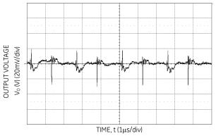
Figure 8. Typical output ripple and noise (Vin = Vin,nom, Io =  $I_{0,max}$ ).
