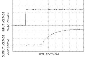
Figure 3. Transient Response to Dynamic Load Change,  $0.1A/\mu S$ , from 75% to 50% to 75% of full load.
