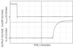
Figure 11. Typical Start-up Using Remote On/Off, negative logic version shown ( $V_{IN} = V_{IN,NOM}$ ,  $I_0 = I_{O,max}$ ).
