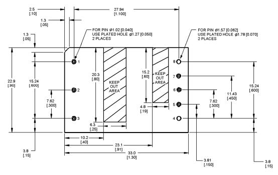
TH Recommended Pad Layout (Component Side View)
