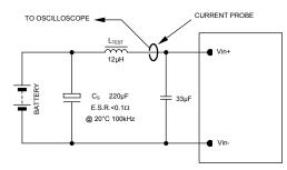
NOTE: Measure input reflected ripple current with a simulated source inductance (LTEST) of 12µH. Capacitor Cs offsets possible battery impedance. Measure current as shown above.
