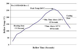
Figure 25. Recommended linear reflow profile using Sn/Ag/Cu solder.
