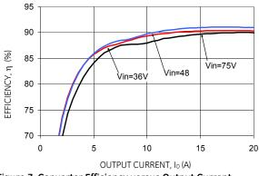
Figure 7. Converter Efficiency versus Output Current.
