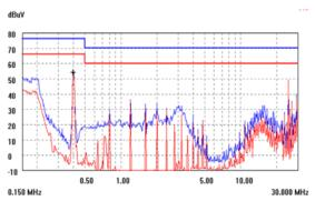
Figure 21. KNW020A0F-88 Quasi Peak Conducted Emissions with EN 55022 Class A limits, Figure 20 filter ( $V_{IN} = V_{IN,NOM}$ ,  $I_o = 0.80 \; I_{o,max}$ ).
