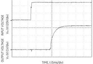
Figure 12. Typical Start-up Using Input Voltage ( $V_{IN} = V_{IN,NOM}$ ,  $I_0 = I_{0,max}$ ).
