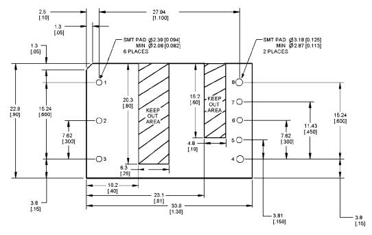
SMT Recommended Pad Layout (Component Side View)
