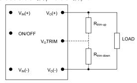
Figure 18. Circuit Configuration to Trim Output Voltage.
