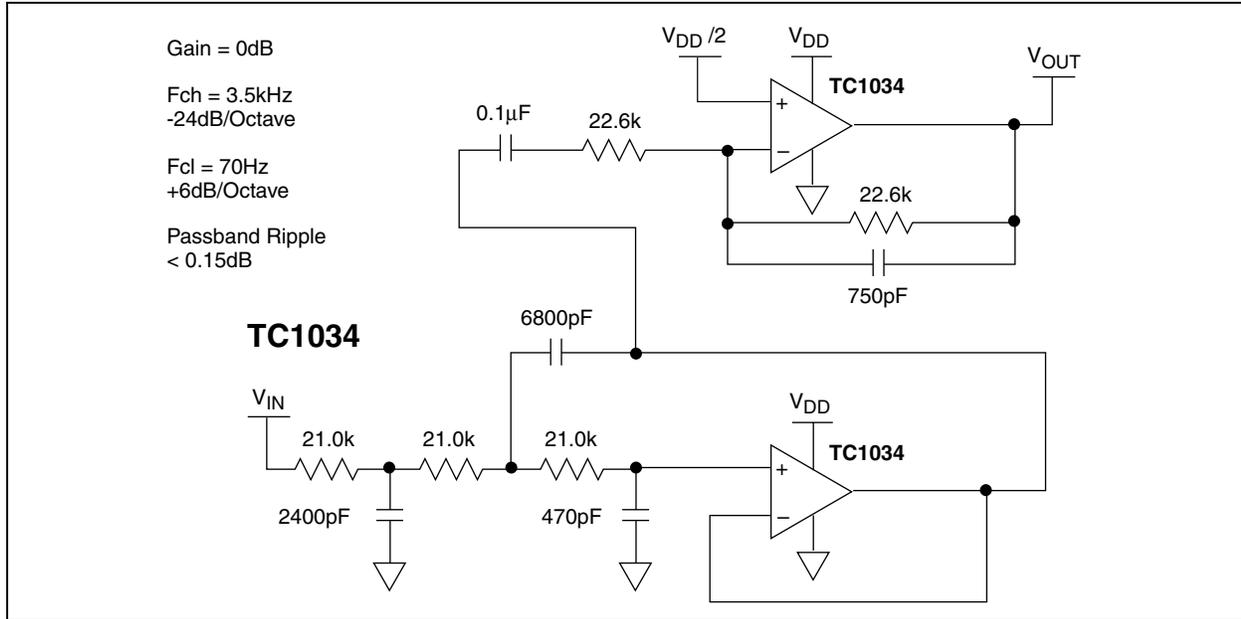
**FIGURE 4-2: SECOND ORDER SAT BANDPASS FILTER**
