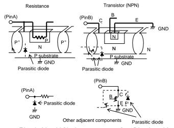
Fig-1 Simplified structure of a Bipolar IC
