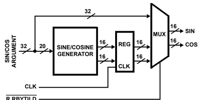
FIGURE 2. SINE/COSINE SECTION
