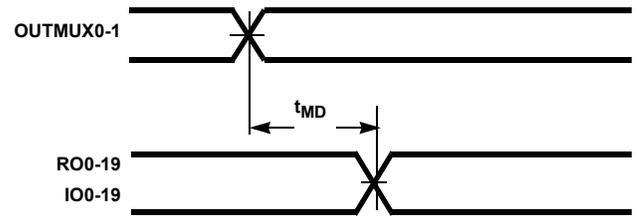
FIGURE 10. MULTIPLEXER TIMING
