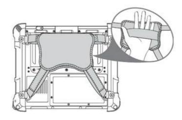
Attach the shoulder strap to the rear of your tablet PC using two screws as shown.
