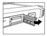
2. Press the SD card inwards to eject it from the slot.
