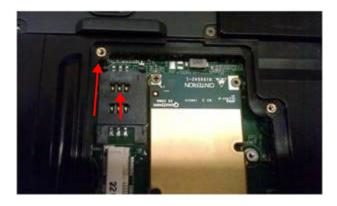
3. Put the SIM card into the slot, with the metallic part facing down until it clicks into place.
