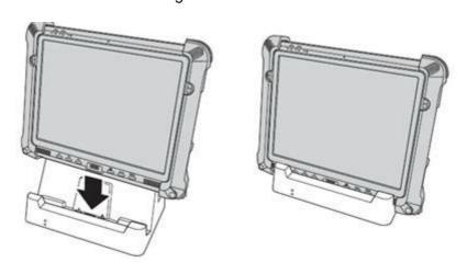
To charge the external battery, attach the battery to the docking stand as shown below.
