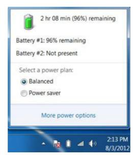
Balanced Automatically balanced performance with energy consumption. Power saver Saves energy by reducing PWS-770's performance.
