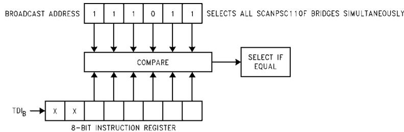
FIGURE 7. Broadcast Addressing: Address Loaded into Instruction Register
