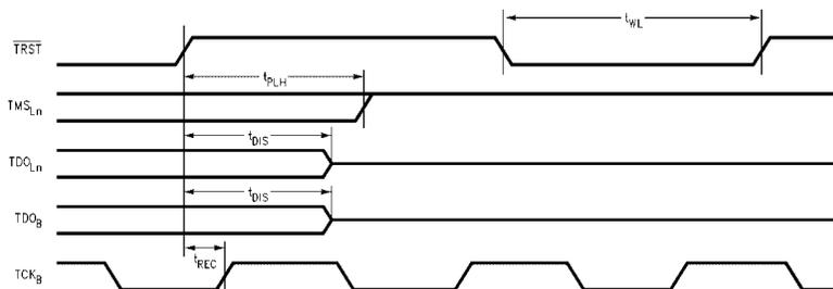
FIGURE 15. Reset Waveforms
