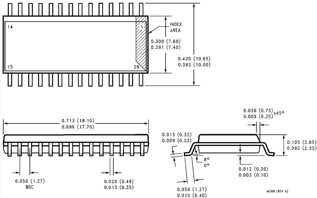
**28-Lead Small Outline Integrated Circuit (SOIC), JEDEC MS-013, 0.300 Wide)
