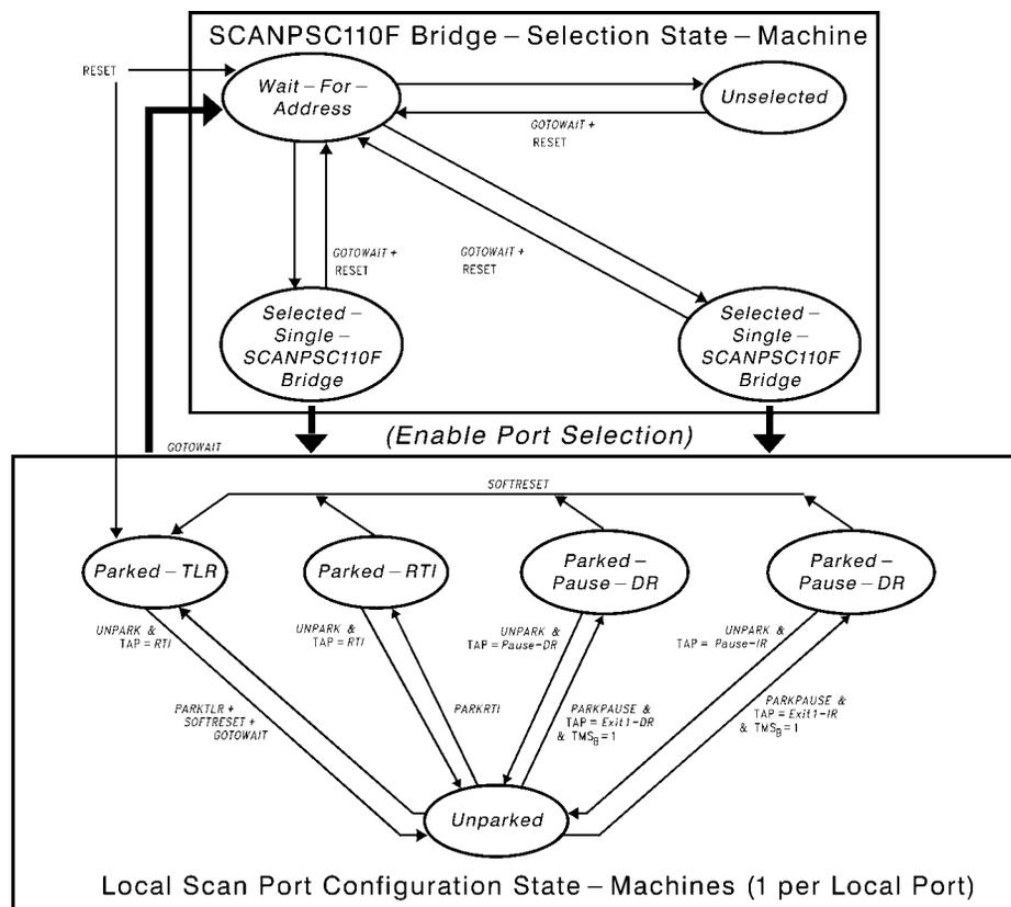
**FIGURE 5. Relationship Between SCANPSC110F Bridge State Machines**
