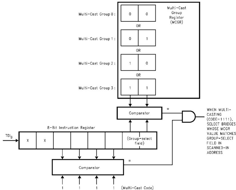
FIGURE 8. Multi-Cast Addressing: Address Loaded into Instruction Register
