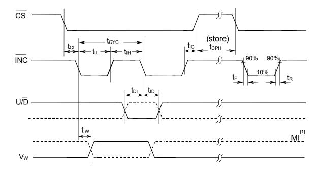
FIGURE 3 -WMS7140/1 TIMING DIAGRAM
