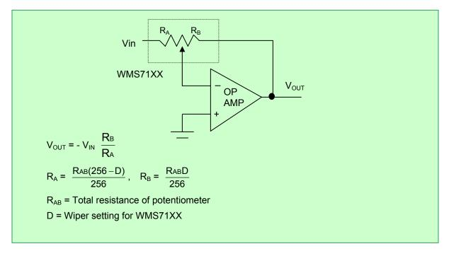
FIGURE 5 - PROGRAMMABLE INVERTING GAIN AMPLIFIER USING THE WMS7140/1
