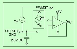
Gain vs. frequency test circuit
