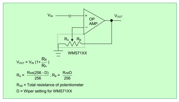
FIGURE 6 - PROGRAMMABLE NON-INVERTING GAIN AMPLIFIER USING THE WMS7140/1
