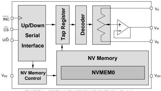
FIGURE 2 – WMS7141 BLOCK DIAGRAM (Divider Mode)
