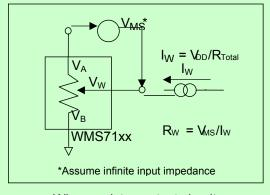
Wiper resistance test circuit
