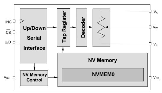
FIGURE 1 – WMS7140 BLOCK DIAGRAM (Rheostat Mode)
