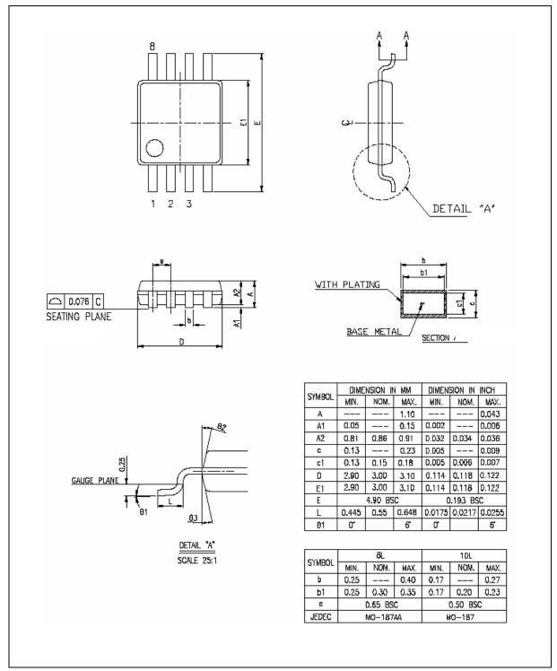
FIGURE 12: 8L 3MM MSOP
