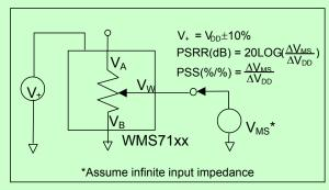
Power supply sensitivity test circuit (PSS, PSRR)
