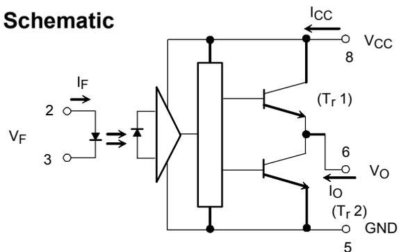
A 0.1 $\mu\text{F}$  bypass capacitor must be connected between pin 8 and 5(see Note 5).
