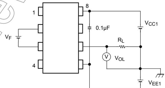
**Test Circuit 5:  $t_{pLH}$ ,  $t_{pHL}$ ,  $t_r$ ,  $t_f$**
