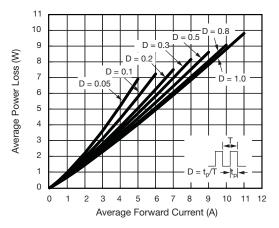
Fig. 2 - Forward Power Loss Characteristics
