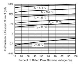
Fig. 4 - Typical Reverse Leakage Characteristics
