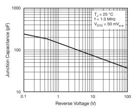
Fig. 5 - Typical Junction Capacitance
