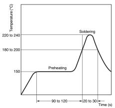
**Note:** The temperature profile indicates the temperature on the circuit board.
