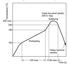
Note: The temperature profile indicates the temperature on the PCB.
