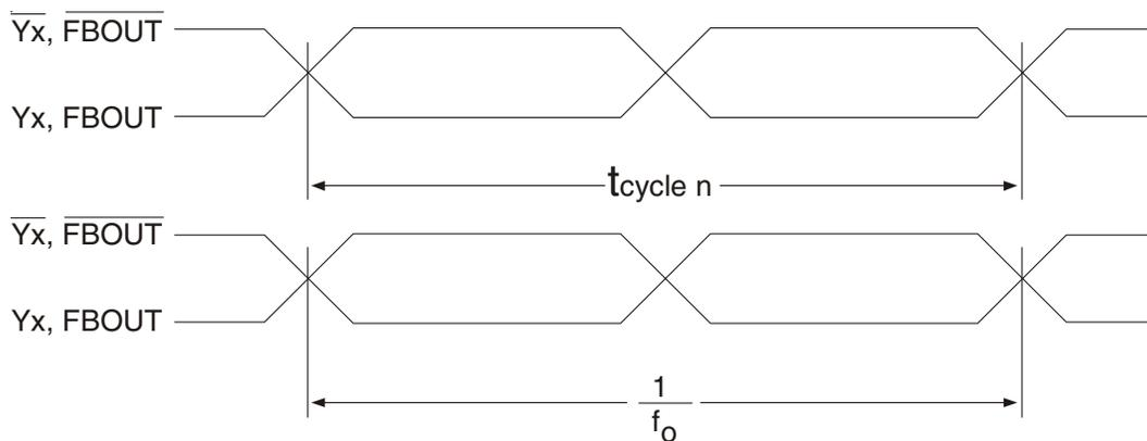
$$t_{jit(per)} = t_{cycle\ n} - \frac{1}{f_0}$$
