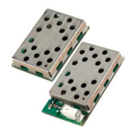
The BTM430 and BTM431 Bluetooth® modules from Laird Technologies have been designed to meet the needs of developers who wish to add robust, short range Bluetooth data connectivity to their products. They are based on the market leading Cambridge Silicon Radio BC04 chipset, providing exceptionally low power consumption with outstanding range.
