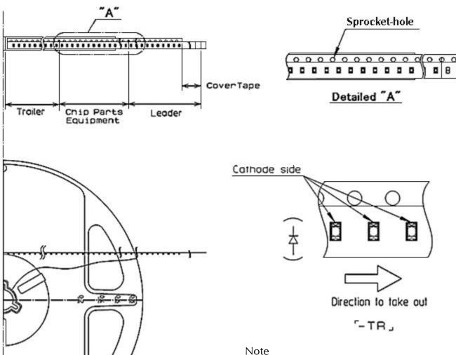
"-TR" means cathode side of LEDs should be placed on the sprocket-hole side.
