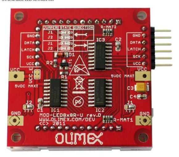
**DESCTIPTION:** MOD-LED8x8 is LED is stackable matrix which allow you to make any size LED array display by stacking them (snap-on) together. It stacks with MSP430-LED8x8-BOOSTERPACK which controll it and with additional MOD-LED8x8 you can make any size LED array display which to control with the low cost MSP430 Launchpad.
