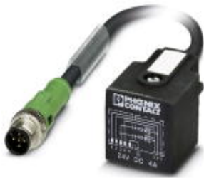
Sensor/Actuator cable, 5-position, PUR halogen-free, Black-gray RAL 7021, Plug straight M12, A-coded, on AD valve plug (pressure switch), with 2 LEDs, Cable length: 1.5 m
