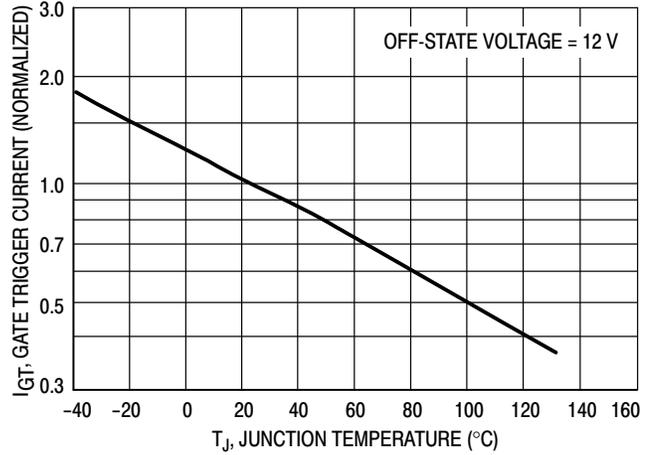
**Figure 7. Typical Gate Trigger Current versus Temperature**
