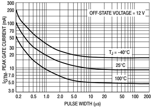
**Figure 6. Typical Gate Trigger Current versus Pulse Width**
