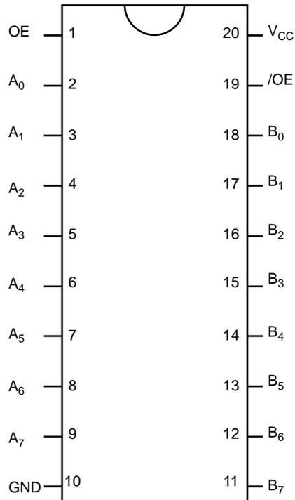
Figure 2. Pin Configuration
