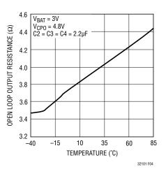
Figure 4. Typical 2x R<sub>OL</sub> vs Temperature
