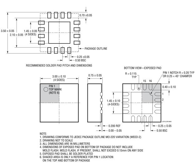
**UD Package** 16-Lead Plastic QFN  $(3mm \times 3mm)$ (Reference LTC DWG # 05-08-1691)
