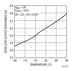
Figure 3. Typical 1.5x R<sub>OL</sub> vs Temperature
