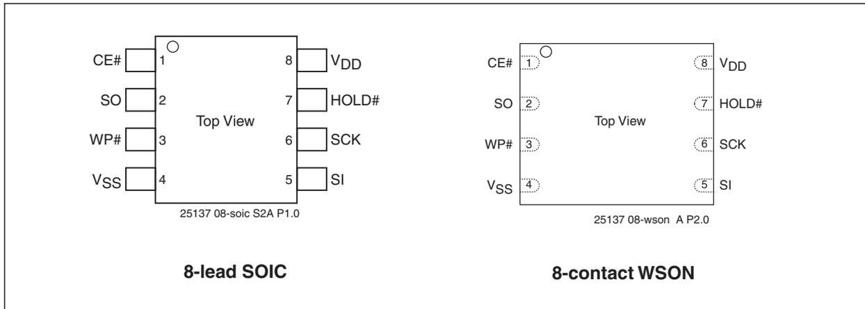
FIGURE 2-1: PIN ASSIGNMENTS
