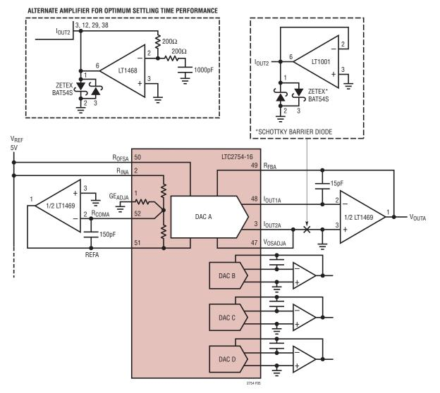
Figure 5. Optional Circuits for Driving  $I_{\text{OUT2}}$  from GND with a Force/Sense Amplifier.
