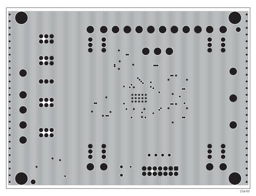
Figure 7. LTC2754 Evaluation Board DC1546. Layer 2, GND Plane
