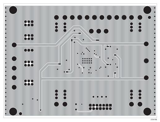
Figure 8. LTC2754 Evaluation Board DC1546. Layer 3, Power Traces
