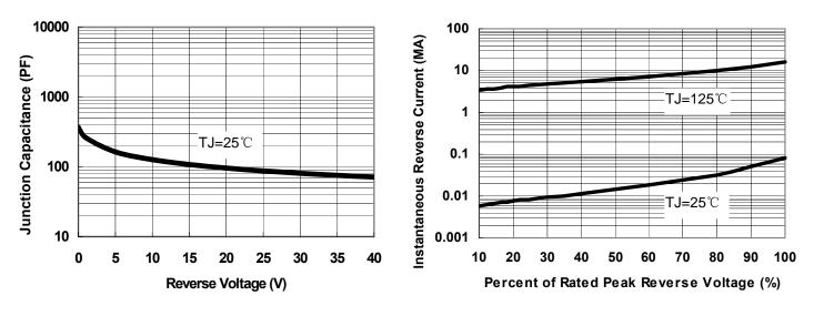
**Fig.1-Typical Junction Capacitance**
