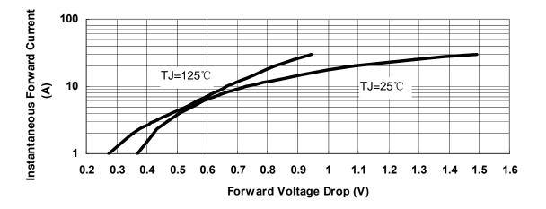
Fig.3-Typical Instantaneous Forward Voltage Characteristics
