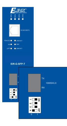
The copper port is 10/100/1000Base-TX and will auto negotiate a connection starting at gigabit speed. High quality Category 5e cable or better should be used. 1000BASE-T requires all four pairs to be present and is far less tolerant of poorly installed wiring than 100BASE-TX systems. A 1000Base-SX/LX SFP module socket for Gigabit optic expansion is located above DIP switch.
