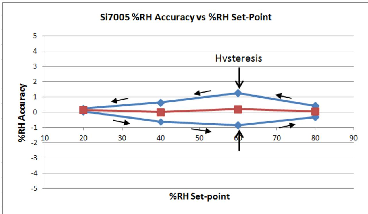
Figure 7. Measuring Sensor Accuracy Including Hysteresis
