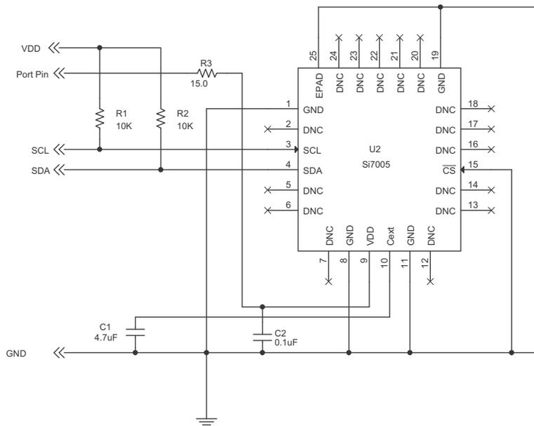
**Figure 5. Typical Application Circuit for Battery-Powered Applications**
