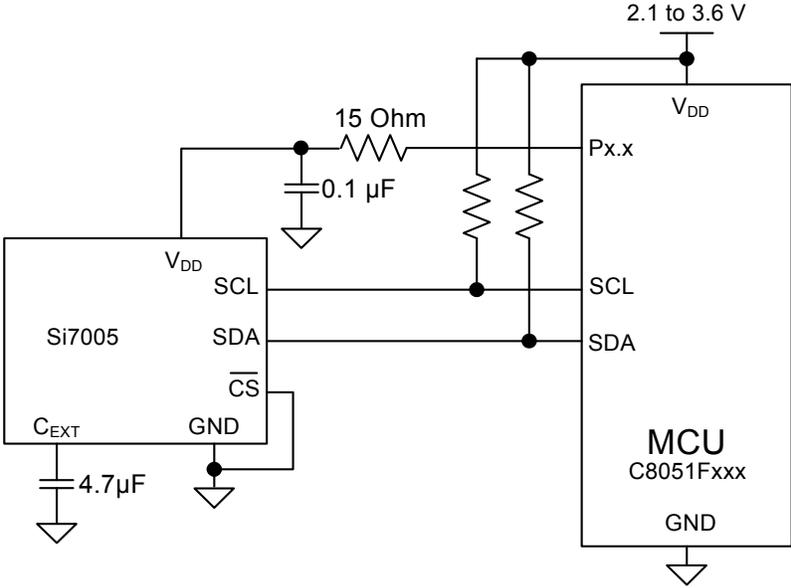
Figure 10. Recommended Connection Diagram for Low-Power Battery Operation
