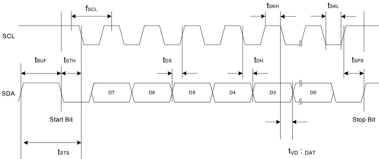
**Figure 1. I<sup>2</sup>C Interface Timing Diagram**
