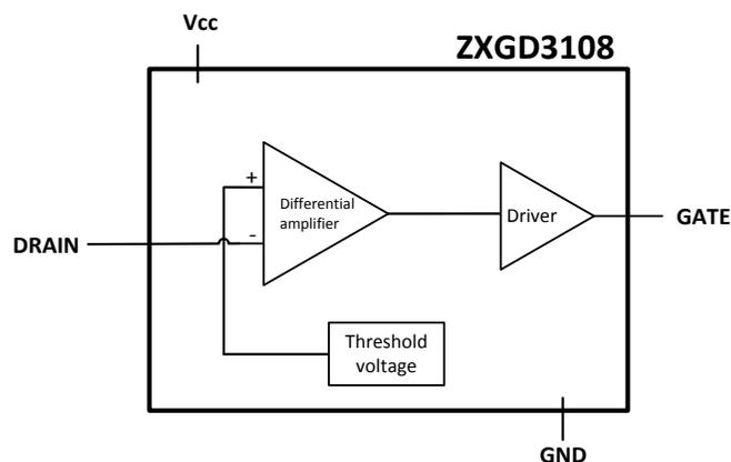
The device is comprised of a differential amplifier and high current driver. The differential amplifier acts as a detector and monitors the DRAIN-to-GND Pin voltage difference. When this difference is less than the threshold voltage ( $V_T$ ), then a positive output voltage approaching  $V_{CC}$  is given on the GATE Pin. Conversely, when the DRAIN-to-GND Pin voltage difference is greater than  $V_T$ , then the GATE Pin voltage is rapidly reduced towards the GND voltage.
