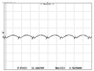
Figure 7: Output ripple & noise at 12Vin, 0.59V/10A out
