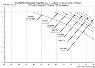
**Figure 30:** Output current vs. ambient temperature and air velocity @ Vin=5.0V, Vout=2.5V(Through PCB Orientation)
