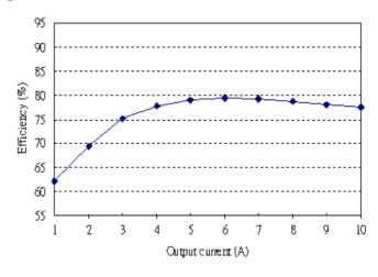
Figure 2: Converter efficiency vs. output current (0.9V output voltage, 12V input)
