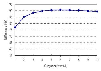
Figure 4: Converter efficiency vs. output current (2.5V output voltage, 12V input)
