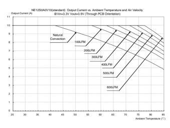
Figure 31: Output current vs. ambient temperature and air velocity @Vin=3.3V, Vout=0.9V(Through PCB Orientation)
