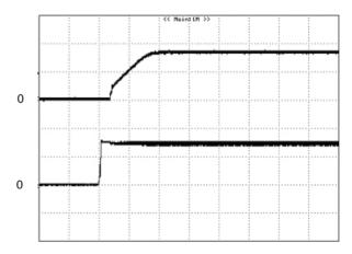
Figure 16: Turn on delay time at Remote On/Off, 3.3V/10A out Ch1: Enable Ch4: Vout
