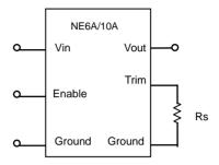
Figure 21: Trimming Output Voltage
