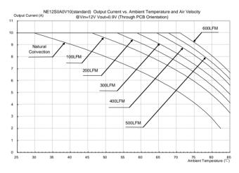
Figure 26: Output current vs. ambient temperature and air velocity @Vin=12V, Vout=0.9V(Through PCB Orientation)
