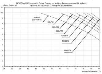
**Figure 29:** Output current vs. ambient temperature and air velocity @ Vin=5V, Vout=0.9V(Through PCB Orientation)
