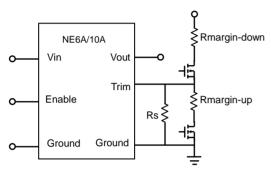
Figure 22: Circuit configuration for output voltage margining
