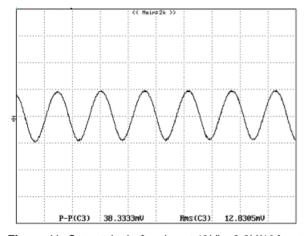
Figure 11: Output ripple & noise at 12Vin, 3.3V/10A out
