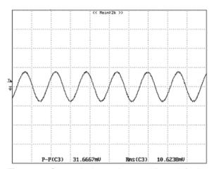
Figure 10: Output ripple & noise at 12Vin, 2.5V/10A out
