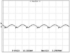
Figure 8: Output ripple & noise at 12Vin, 0.9V/10A out
