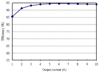
**Figure 6:** Converter efficiency vs. output current (5.0V output voltage, 12V input)
