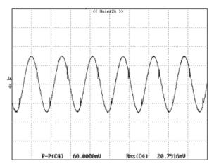
Figure 12: Output ripple & noise at 12Vin, 5.0V/10A out
