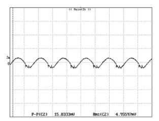
Figure 9: Output ripple & noise at 12 Vin, 1.8 V/10 A out
