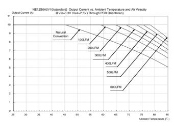
Figure 32: Output current vs. ambient temperature and air velocity @Vin=3.3V, Vout=2.5V(Through PCB Orientation)
