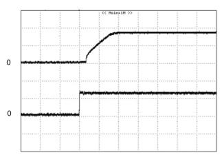
Figure 13: Turn on delay time at 12Vin, 1.0V/10A out Ch1: Vin Ch4: Vout
