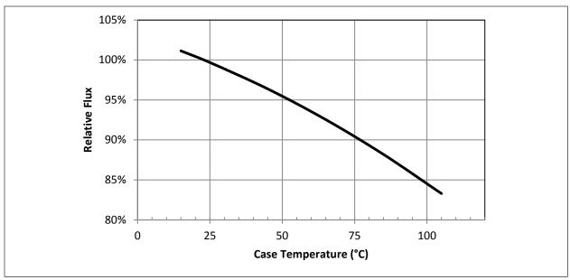
Figure 4: Typical DC Flux vs. Case Temperature
