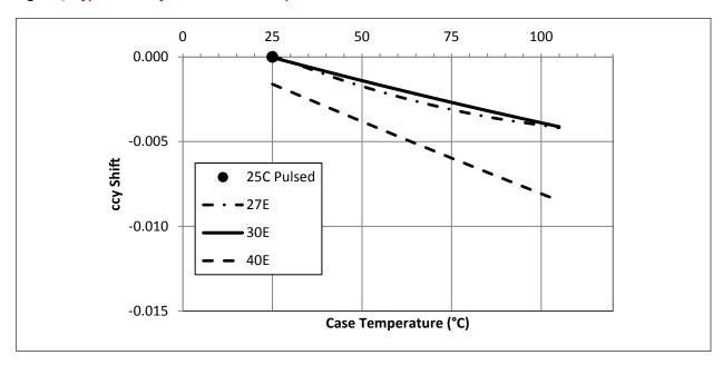
Figure 6: Typical DC ccx Shift vs. Case Temperature
