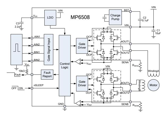
Figure 1: Function Block Diagram
