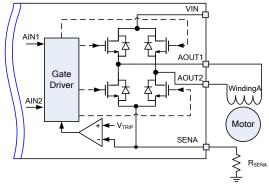
Figure 2: Full-Bridge Control Circuit
