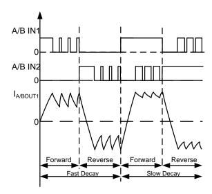
Figure 5: External PWM Current Control Waveform
