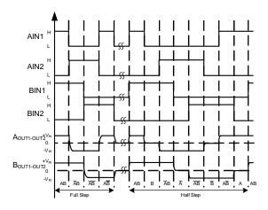
Figure 7: Signal Logic Sequences for Full-Step and Half-Step
