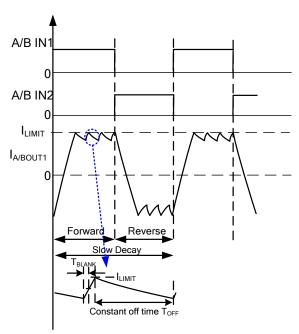
Figure 6: Internal PWM Current Control Waveform Sleep Mode
