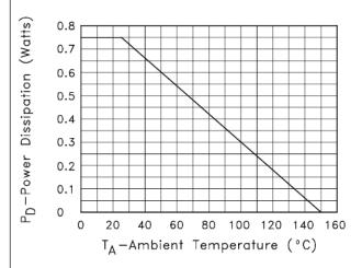
FIG. 10 Power vs. Temperature Derating Curve (Ambient)
